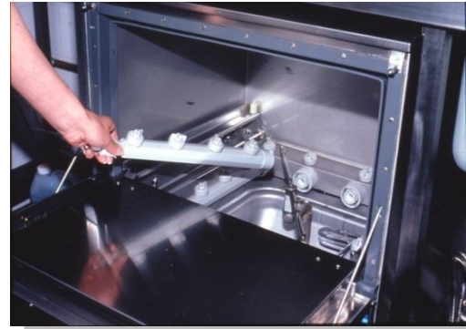
Check wash and rinse arms
