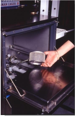
Check and clean filters
